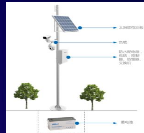
Solar power supply
